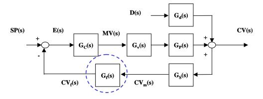
Clearly, the filter is in the feedback loop. In addition, the filter appears in the characteristic equation, as shown in the following transfer function.
