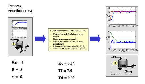
We will evaluate the stability, i.e., the gain margin, without and with a filter. The Bode stability analysis gives the following results with the tuning in the figure and no filter.
