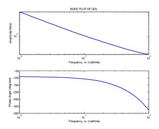
The critical frequency is between 0.41382 and 0.41477 The amplitude ratio at the critical frequency is 0.32213
