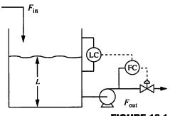
FIGURE 18.1 Typical level control system.
