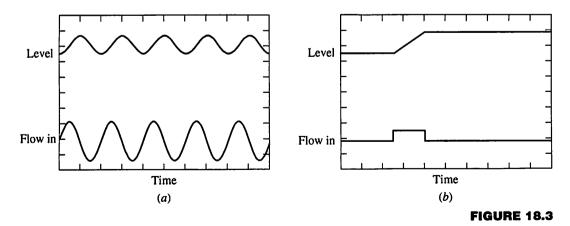
Response of a non-self-regulating level without control: (a) to sine flow variation; (b) to a pulse flow variation.
