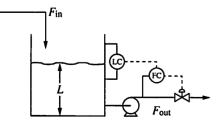
**Solution.** The nonlinear controller requires two additional parameters. The guidelines suggest that  $r_{\kappa} = 20$ , and we select  $L'_{B}$  to be relatively large, to provide small outlet flow variations for most inlet flow oscillations. Thus,  $L'_{B} = 0.7$  m, which is  $\pm 35\%$  of the level range. For the PI controller,
